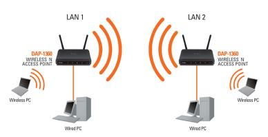
Connecting two separate LANs together through two DAP-1360 units (Wireless PCs can access the DAP-1360 units)
