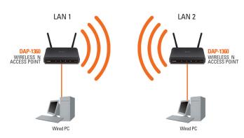
Connecting two separate LANs together through two DAP-1360 units (Wireless PCs cannot access the DAP-1360 units)
