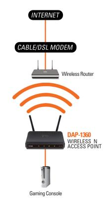
Ethernet-enabled gaming console using the DAP-1360 as a wireless interface to access the Internet
