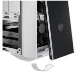
Easy fan installation without removing the full front bezel, but simply by removing the front panel
