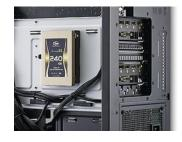
SSD can also be installed behind the motherboard tray
