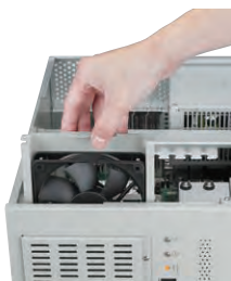
Easy-to-maintain cooling fan
