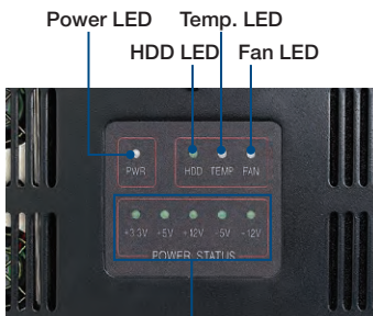
Power voltage status
