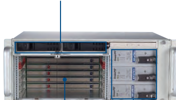
Two hot-swappable SATA HDD bays
