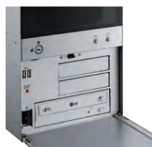
Dual External 3.5" SAS/SATA HDD trays
