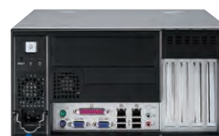
Plug ring-lock securely fastens the power cord
